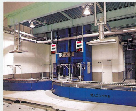
びん受入コンベヤ [垂直コンベヤ] (2系列) Glass bottle receiving conveyor [Vertical conveyor] (2 lines)
